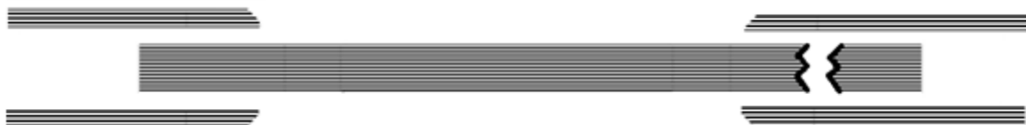
Dog ears shearing off a carbon fibre dog bon specimen, leading to failure in the grips
