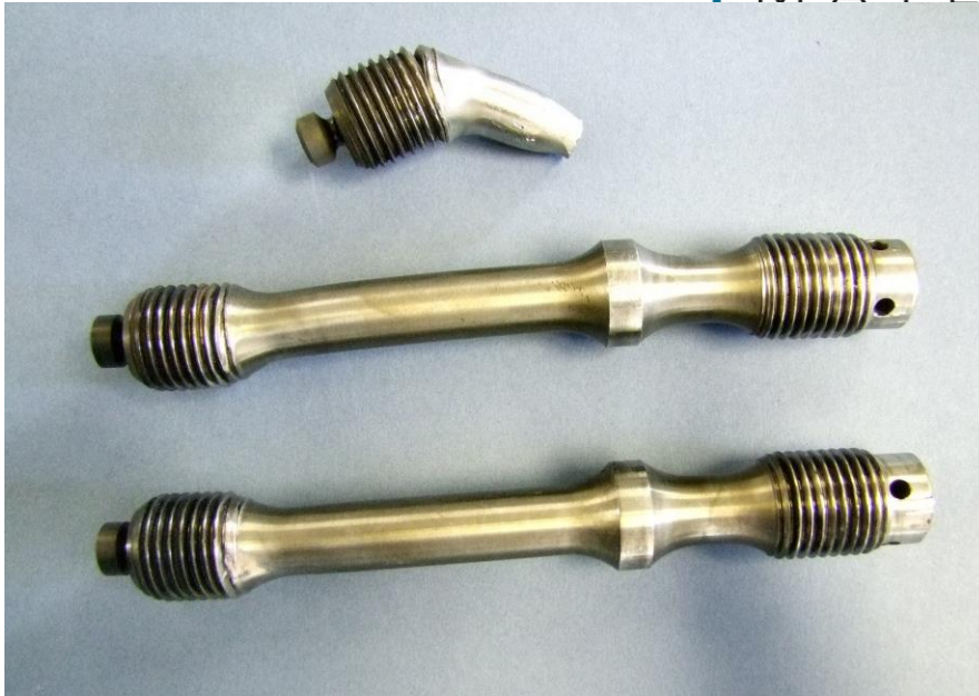
Figure 3.1 Piston crown studs after removal
