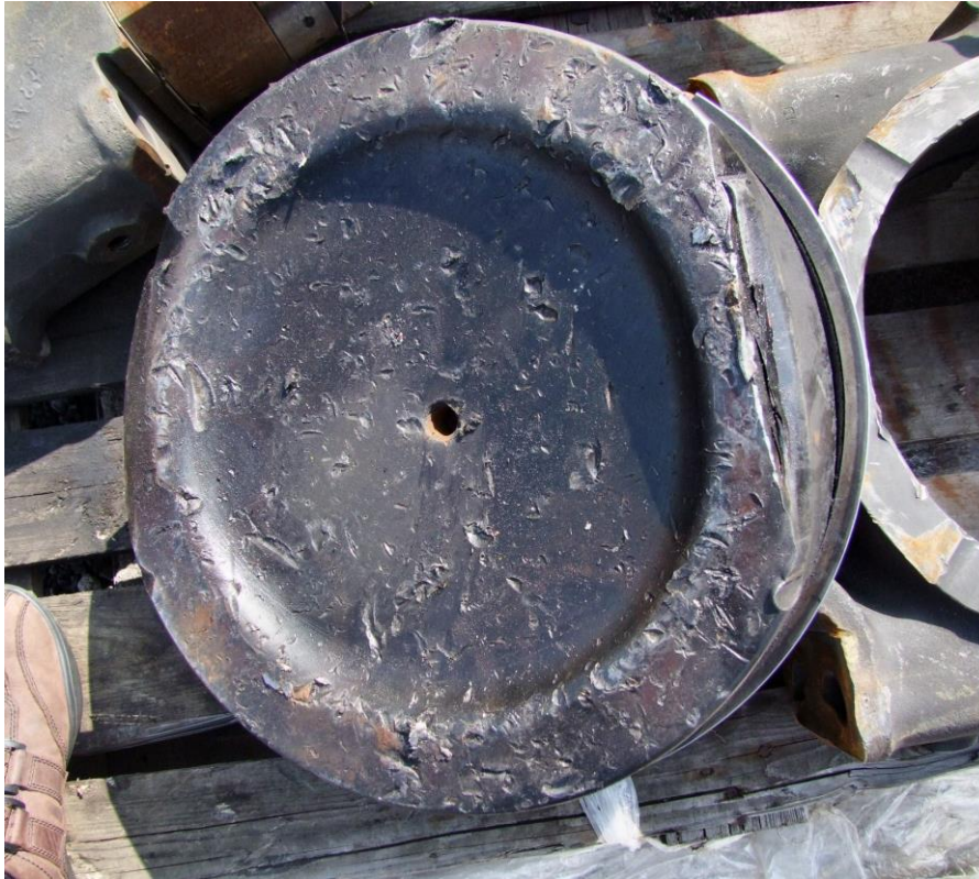
Figure 2.1 Piston working face
