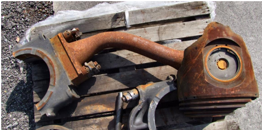
Figure 2.4 Bent conrod, part of big end, and lower part of piston
