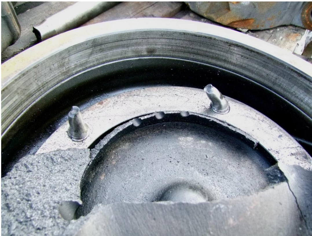
Figure 2.8 Piston crown studs 1 and 2
