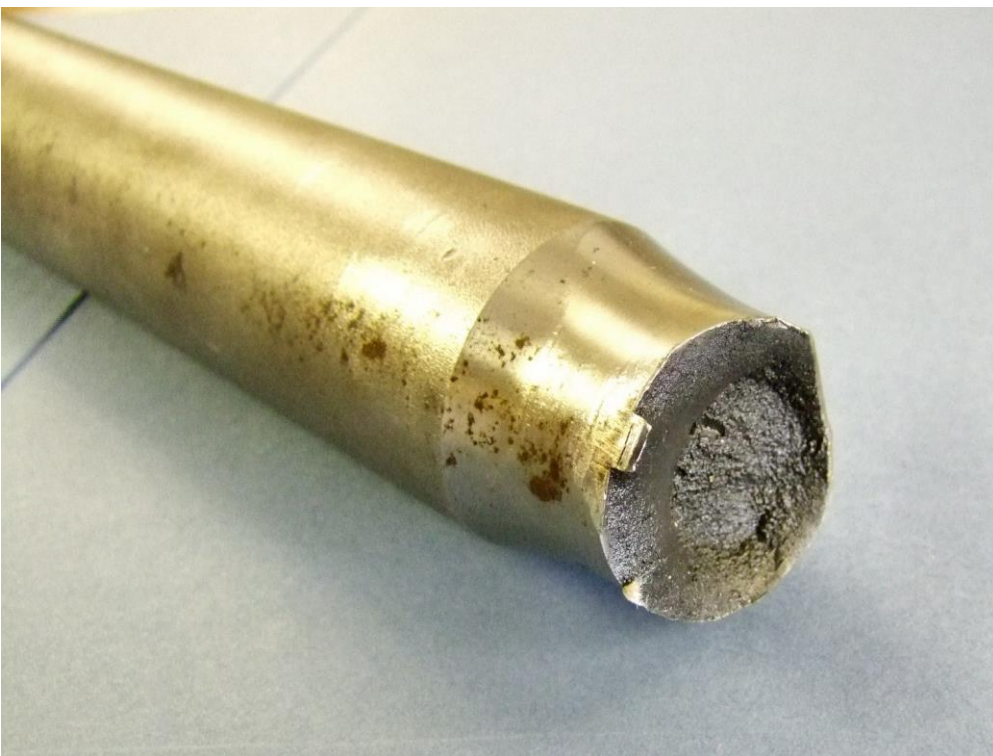
Figure 3.9 Big end bolt showing the fracture face
