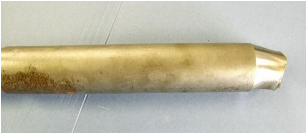
Figure 3.8 Big end bolt with tensile / bend type failure
