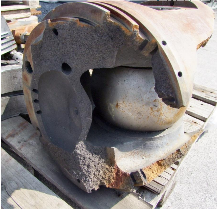
Figure 2.3 Lower part of piston - fracture face
