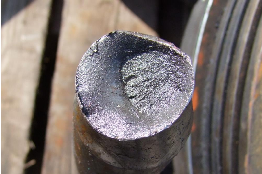
Figure 2.7 Big end bolt fracture face
