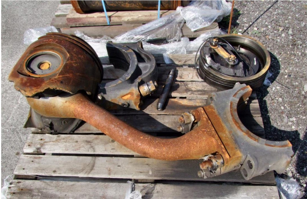
Figure 1.1 Conrod, piston and bolt as received
