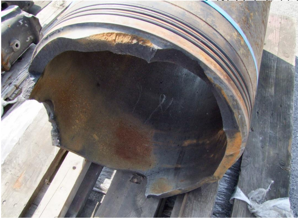
Figure 2.5 Fractured end of cylinder liner
