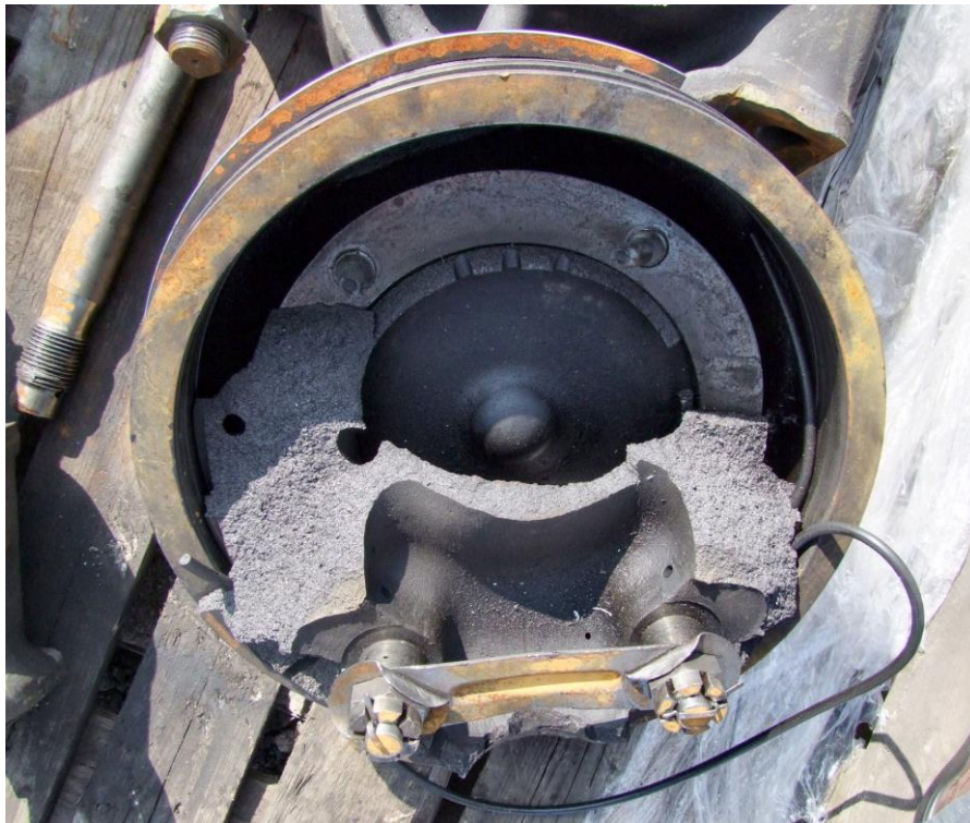
Figure 2.2 Top piece of piston, showing the underside fracture face
